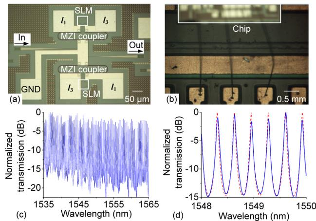
Fig. 4. (a), (b) Micrograph of (a) the fabricated device and (b) the device after wire-bonding to a PCB. (c) Measured transmission spectrum of the comb filter in the wavelength range from 1535 nm to 1565 nm. (d) Measured (blue-solid curve) and fitted (red-dot curve) transmission spectra in the wavelength range from 1548 nm to 1550 nm. SLM: Sagnac loop mirror. MZI: Mach-Zehnder interferometer. PCB: printed circuit board.
