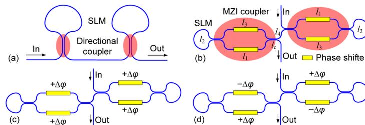
Fig. 1. (a) A FPI comb filter consists of two loop mirrors. (b) Schematic of the proposed comb filter based on SLMs with MZI couplers. (c) Common and (d) differential tuning of the MZI couplers for wavelength and bandwidth tuning of the comb filter, respectively. SLM: Sagnac loop mirror. MZI: Mach-Zehnder interferometer. FPI: Fabry-Perot interferometer.
