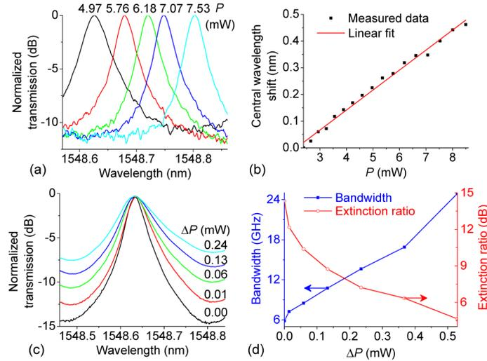
Fig. 5. (a), (c) Measured transmission spectra of (a) central wavelength and (c) bandwidth tuning versus heating power  $P$  of each micro-heater and differential heating power  $\Delta P$ , respectively. (b) Central wavelength shift versus heating power  $P$  of each micro-heater. (d) Bandwidth and extinction ratio versus differential heating power  $\Delta P$ .
