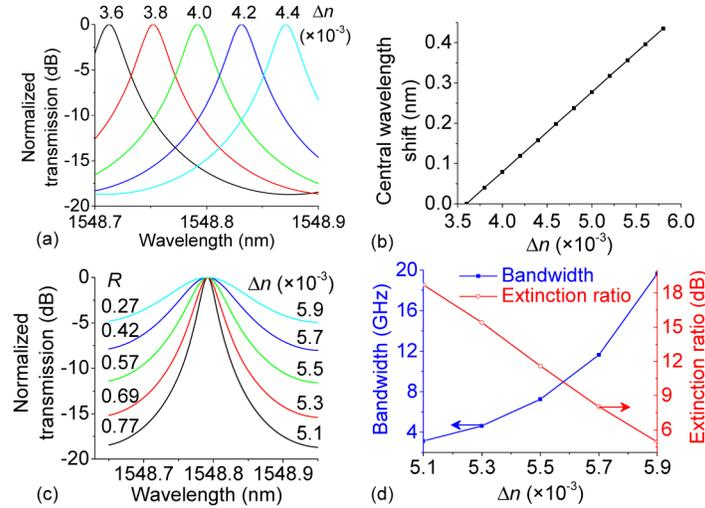
Fig. 2. (a), (c) Simulated transmission spectra of (a) central wavelength and (c) bandwidth tuning by changing the refractive indexes of the phase shifters along the MZI arms according to Figs. 1(c) and 1(d), respectively. (b) Central wavelength shift versus  $\Delta n$ . (d) Bandwidth and extinction ratio versus  $\Delta n$ .  $\Delta n$ : refractive index change.  $R$ : reflectivity.
