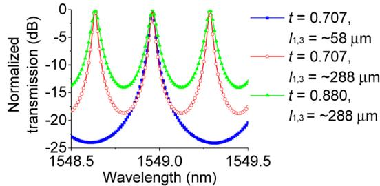
Fig. 3. Simulated transmission spectra of the comb filter with different  $t$  and  $l_{1,3}$ .
